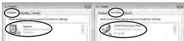
In the "Sound" window, verify that "ZOOM S2t C5.1t Audio" is listed under the Play and Record devices and that the device is checked. (To switch between Play and Record, click the tabs at the top of the window.)
