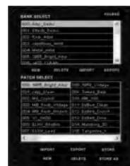
You can start up "Patch Manager" with [PATCH] button. Here you can select/operate the patches.
