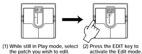
Immediately after entering Edit mode from Play mode, the topmost parameter cursor indicator (PRE DRIVE) flashes, and the setting of this parameter is shown on the display. The flashing parameter cursor always indicates which parameter is selected for editing.
