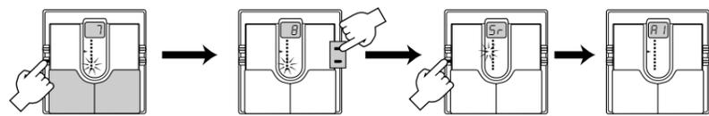
\* Use the VALUE +/- keys to change the setting of the parameter. For details on parameters, please refer to section 12 "Effect Parameters".
