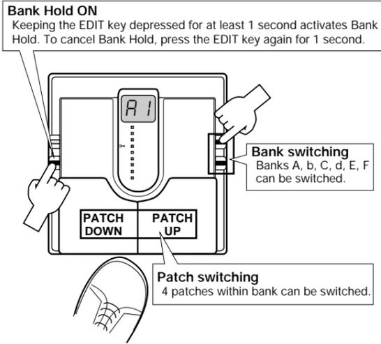
Bank/patch switching when Bank Hold is on
