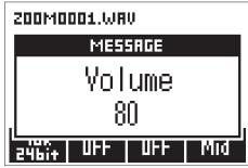
While checking the audio level meter of the other device, adjust the audio signal level so that it never exceeds –6 dB.
