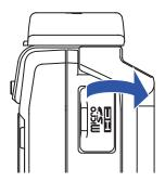
2. Insert the microSD card into the card slot.
