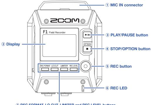
7 REC FORMAT, LO CUT, LIMITER and REC LEVEL buttons
