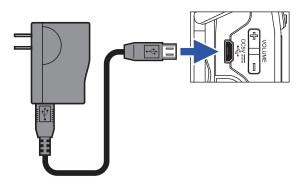
2. Plug the AC adapter into an outlet.
