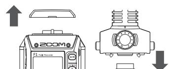
2. While pressing the buttons on the sides of the mic capsule, connect it to the **F1**, inserting it completely.
