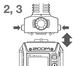
3. To disconnect the mic capsule, pull it away from the unit while pressing the buttons on its sides.
