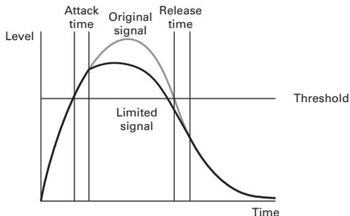
When the limiter is ON, if the input signal level exceeds the set threshold value, the signal level will be suppressed to prevent the sound from distorting.
