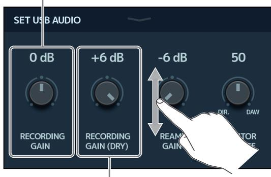
This adjusts the recording level of signals before effect processing.
