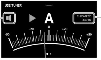
This shows the tuner type and standard pitch. Touch this to open the SET TUNER screen. (See below.)
