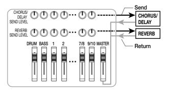
The amount of signal sent to each effect (send level) adjusts the depth of each send/return effect for each channel. Raising the send level will increase the amount of signal that is sent to the effect, producing a deeper effect for that channel.
