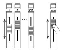
Immediately after the demo song (project) has been loaded, the volume of each track and the overall volume of the entire song will be set automatically, without regard to the current physical positions of the faders. When you operate a fader, the volume will immediately be set to the new position of the fader.
