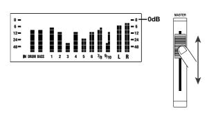
When you have finished adjusting the MASTER fader, press the STOP [] key to stop, and then press the ZERO [III] key to return to the beginning of the song.
