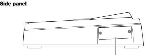
This slot is for installation of a separately sold SCSI board or USB board (planned for release).
