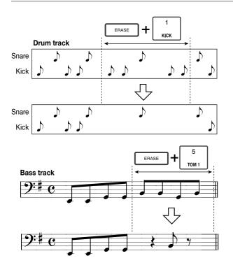
If you want to erase the performance of all pads from the track, hold down the [ERASE] key and press the status key of the corresponding track (DRUM or BASS).
