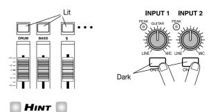
If the INPUT 1/2 [ON/OFF] keys are turned on, any instruments connected to the [INPUT 1/2] jacks can also be mixed.
