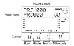
The screen that appears first when the power is turned on is called the "main screen." The main screen is the starting point for all operations.
