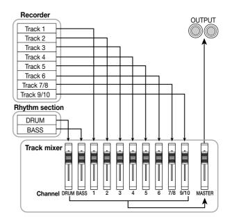
In the track mixer, the signals that are output from each track are handled in units called "channels." The parameters that can be adjusted for each channel (DRUM, BASS, 1 - 6, 7/8, 9/10) are listed in the table below.
