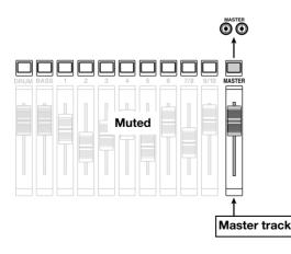
In the MRS-1044 series, one master track can be used per project. Like ordinary tracks, the master track also comprises 10 V-takes. This lets you create multiple versions with a different mixing balance, and select the best V-take later. A master track recorded in this way can be used as source material for creating an audio CD. (The selected V-take of a master track in a project can be written to CD-R/CD-RW.)
