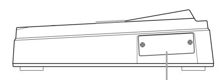
This slot is designed for installation of a separately available SCSI board or USB board.
