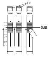
The drum sound and bass sound of the rhythm section are sent respectively to the DRUM channel and BASS channel of the mixer. The DRUM/BASS status keys switch channelmuting on/off, and the DRUM/BASS faders adjust the volume of each channel.
