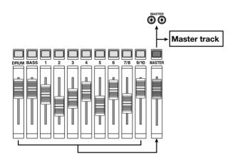
When the master track is played, the signal is inserted just before the MASTER fader. (At this time, the DRUM, BASS, 1 - 6, 7/8, and 9/10 channels are muted.) The MASTER fader can be used to adjust the volume, and the signal can be monitored at the [OUTPUT] jacks.
