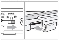
2 2) Insert an SD card (write-protect unlocked) into the slot.
