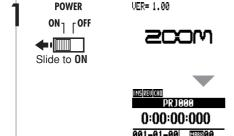
Then turn the power ON for connected instruments and for the monitoring system in that order.
