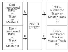
Inserting the insert effect on 8 inputs (8xComp EQ algorithm)
