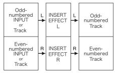
Inserting the insert effect on a stereo input (Stereo, Mastering algorithms)
