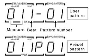
**STEP 2** Use the [UP/DOWN] keys to select the desired pattern number.
