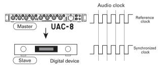
The **UAC-8** is operating as the master, and the audio clock of the **UAC-8** and the other digital device are synchronized.
