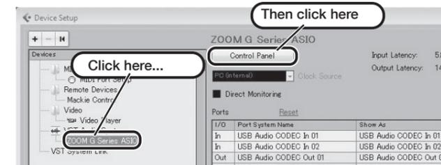
The window that appears lets you set the latency and sampling frequency for the ASIO driver. The latency should be set to a value that is as low as possible without causing sound dropouts during recording and playback.
